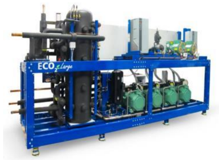
CO2 transcritical power rack for medium-large stores with integrated FTE2.0 and ETE
